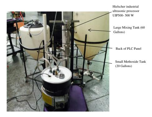
Figure 3. Modified processor with ultrasonictransducer (back of the processor with the ultrasonic unit assembled)
