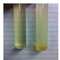
Figure 4. A passed 27/3 test using ultrasonication (left) and a failed test using conventional stirring (right)
